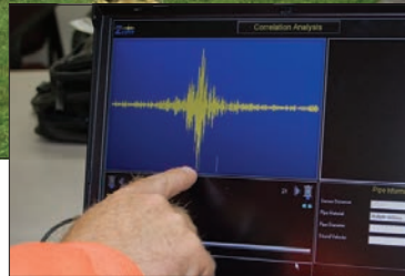
A water leak is viewed using the ZCorr leak detection system from Itron.
